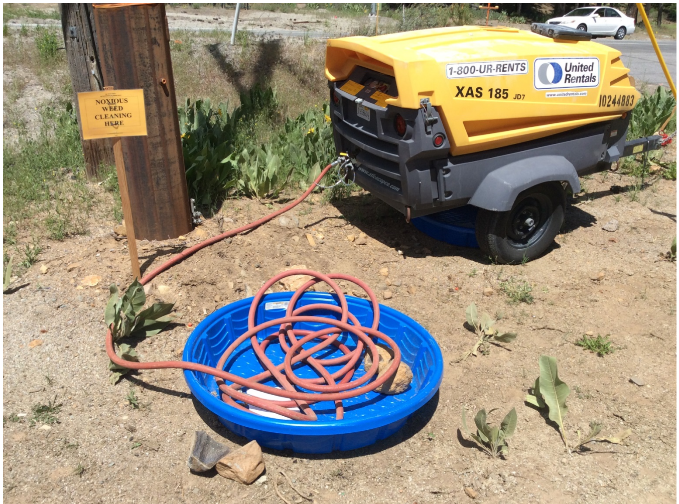
Photo 2: High-pressure air noxious weed cleaning station at ROW access road entrance (APM-BIO-6).
